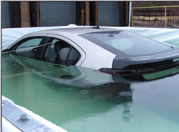
Immersive Saltwater Testing
