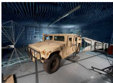
EMI/EMC Testing of a Battery as Installed in a System
